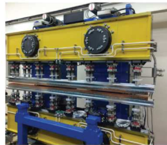
Installation undulator in 3 GeV ring
