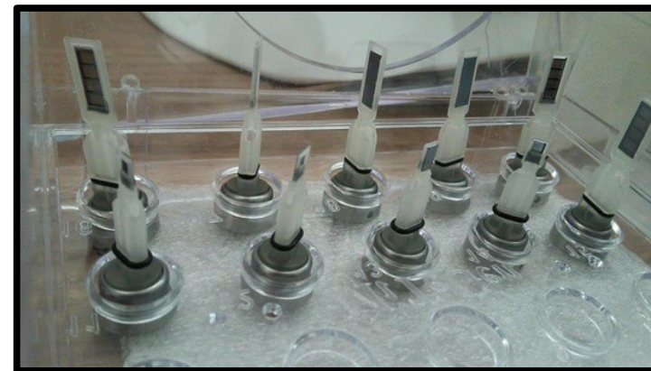
Fixed targeted pins (first tests) and microfluidics sample holders (in collab with Gothenburg University)
