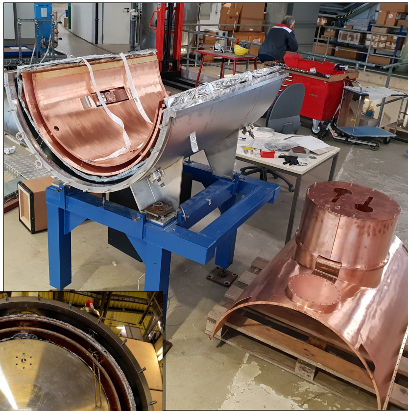
7 Tesla Wavelength Shifter built by Budker Institute, Novosibirsk, Russia
