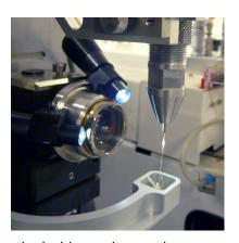
Injector filled with 30  $\mu l$  grease mixed with protein crystals.
